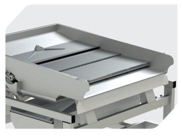
The vibrating hopper offers various benefits. The first is to control the accuracy of the adjustments made to the destemming head. The second is to distribute the harvest evenly over the entire surface of its grid in order to effectively sift out the juice and any small unwanted debris. The third is to orientate the flow of matter horizontally in order to facilitate and optimise the work of the Viniclean rollers.
