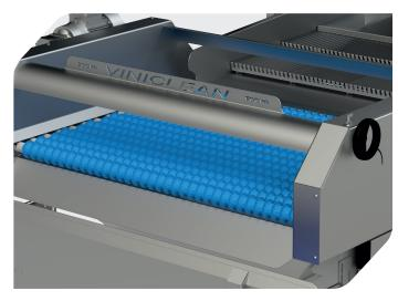
This 15-roller sorting tool, equipped with flexible plastic sleeves with adjustable spacing on two axis, allows for the precise extraction of vegetation and any other debris larger than the grape berry (stems, petioles, leaves, snails, pieces of stump, etc.).
