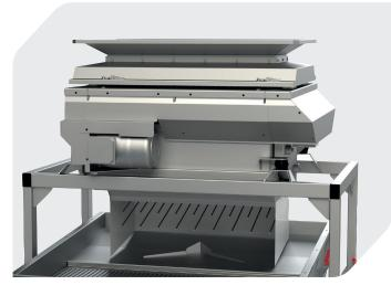
This system, which is unique on the market, allows for a gentle and silent destemming of the harvest by removing the grapes from the stems without the slightest of trauma to the components of the cluster. It consists of two rows of plastic destemming fingers which form a vertical vibrating corridor in which the clusters are guided (1).
