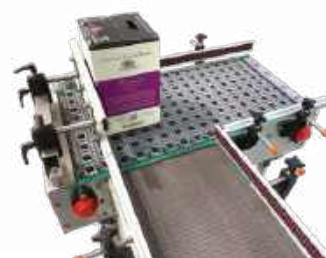
90° Corner for Carton Conveyors
