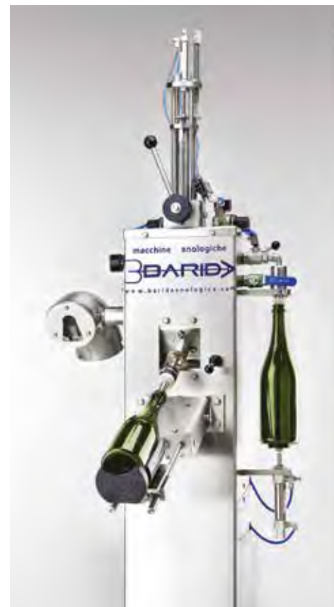
Atlas M Disgorging, Dosage and Levelling Ideal for small producers. Semi-auto disgorging & dosage levelling.
