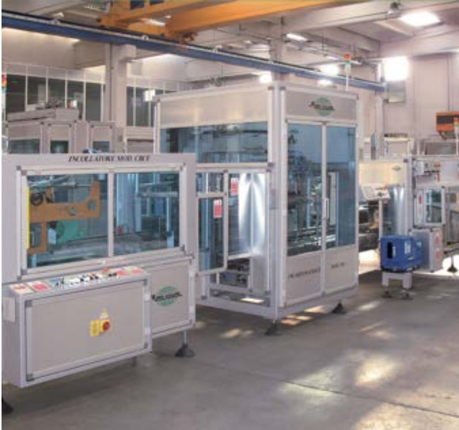
Divisions Inserter. Model 2000/E Suitable to pick-up, open and insert automatically solid carton divisions into cases.
